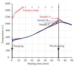
Fig.3. Temperature variation in the bottom of pellet bed.
