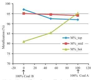
**Fig.7.** The specific portion metallization % with different amount of coal type.
