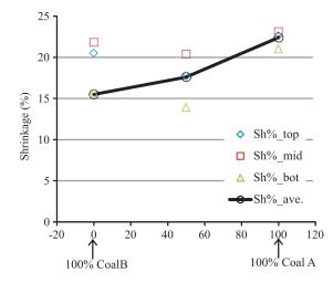
**Fig.5.** The specific portion and whole sample shrinkage % averaged by every individual DRI with different amount of coal type.
