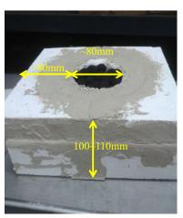
Fig.2. The picture of crucible loading with the green balls.
