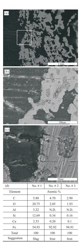
**Fig.6.** SEM images and EDX analysis of sample A on the top layer DRI. (a) Low magnification image taken by near the surface of DRI. (b) Middle magnification image enlarged from the marked area in (a). (c) Middle magnification image zoomed in on the edge of DRI surface. (d) EDX analysis at the points in (b) and (c).
