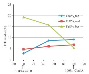
**Fig.10.** The FeO residue % plots in specific portion with different amount of coal type.
