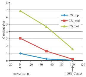
**Fig.9.** The carbon residue % plots in specific portion with different amount of coal type.
