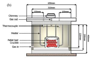
**Fig.1.** (a) The picture and (b) the schematic diagram of the experimental apparatus.
