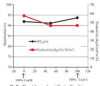
**Fig.8.** The whole sample metallization % and iron productivity with different amount of coal type.
